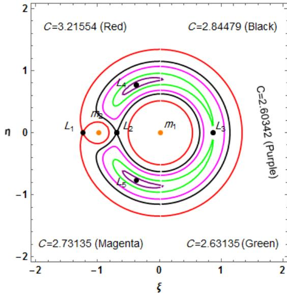
Figure 6(f): Zero velocity curves with mass reduction factor ( $q_1 = 0.75, \sigma_1 = 0.00196, \sigma_2 = 0.105$ ).
